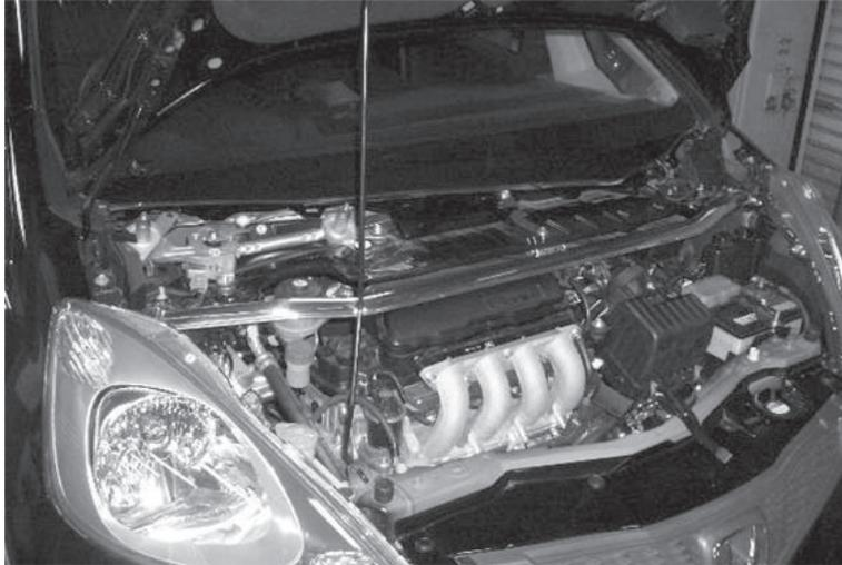
11.) If the strut bar makes contact with the air duct hose, trim the area indicated in the photo.
