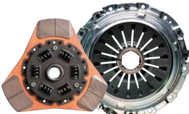
Set of metal clutch disc + clutch cover
