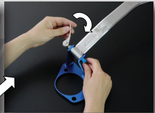
Rotate lever until snug and lock the lever down.
