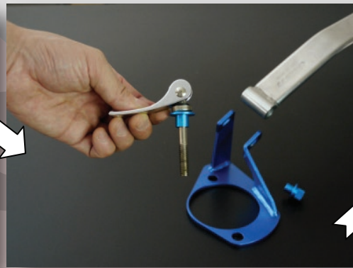
Insert Quick Release Lever and hand-tighten.
