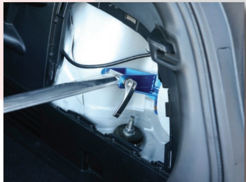
Insert Quick Release Lever and hand-tighten.
