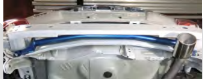
POWER BRACE REAR END
