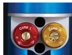
Dial for high speed and low speed bump damping force adjustment
