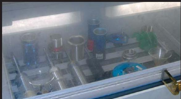
High concentration saltwater direct injection test
