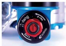
Dial for high speed and low speed bump damping force adjustment
